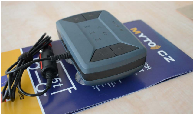
On-board unit for a satellite toll system
