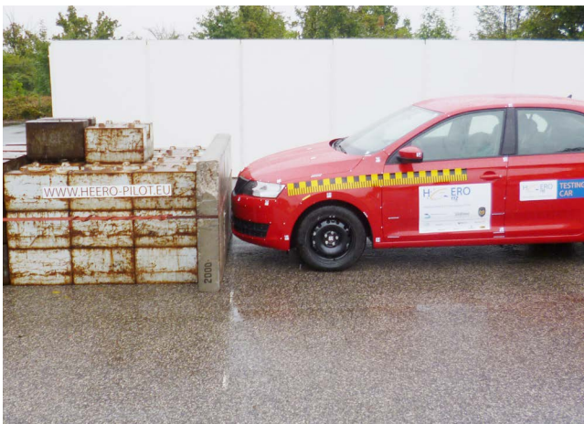
The first CRASHTEST trial deployment of the eCall system (HeERO project for the Ministry of the Interior conducted by the Faculty of Transportation Sciences of the Czech Technical University, Department of Vehicle Technology)
